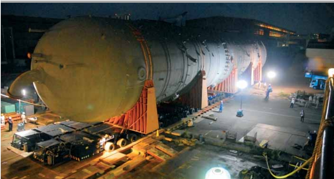
One of the low-temperature FT reactors for the EGTL plant, being shipped from Yokohama, Japan to Escravos, Nigeria.
